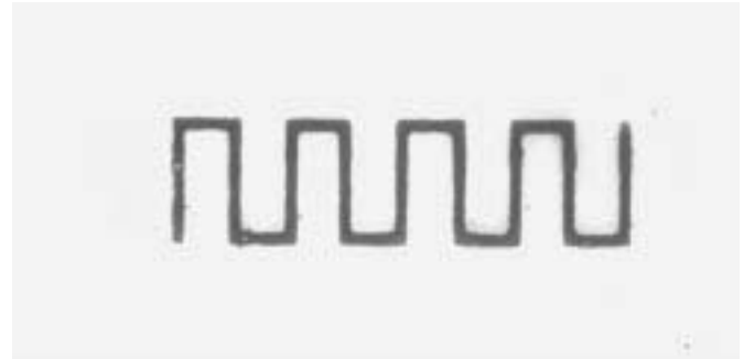
Fig. 5. Screen-printed magnetic polymer composite (80% by volume) with 250- \mu\text{m} features.
